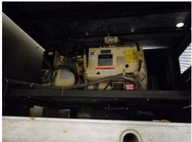
Figure 18 Fire Truck Generator
